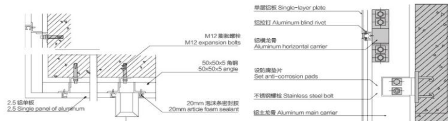
INTERNAL CORNER INSTALLATION ILLUSTRATION TO ALUMINUM SINGLE PLATE 铝单板内部转角安装实例
