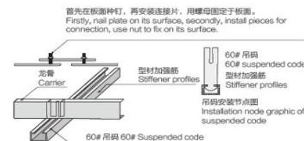
GRAPHIC ILLUSTRATION CONNECTION POINT OF PLATE TO PLATE 板与板连接节点图
